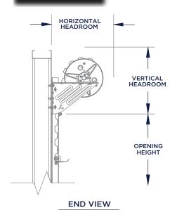
Universal mount 2.25" deep 16-gauge galvanized steel guides require no pre-installation modifications for wood, steel, concrete or filled masonry block applications.
