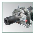
A cam-action spring tension holding device allows quick, easy and equal adjustment of the tension on all springs simultaneously from one end of the door. The cam tensioner bites into the axle helping to eliminate the unwanted spinning of the axle during the initial spring loading or adjustment process.
