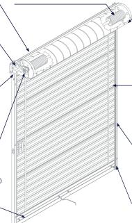
Full width galvanized steel **BARREL** totally encloses the drums, springs and axle. Barrel-type construction reduces door sag, eliminates drum dents and improves operation due to an even support of the curtain for the entire width.
