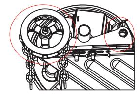
Insert the hoist shaft into the anchor bracket section. Rotate to engage with hex shaft in the drive unit. (Parts removed for clarity.)
