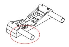
Carefully insert the two tubes of the assembled bracket into the corresponding sections of the drive nuit.
