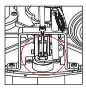
Reinstall knurled split nut and tighten.
