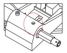
Place the cast iron chain wheel and nylon guide on hoist shaft and retain with cotter pin. Cut hand chain to length and fit to chain wheel.
