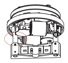
Ensure that maximum penetration of the tubes into the drive unit is achieved.
