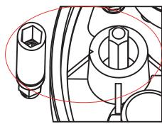
Locate the shaft in position with set screw, ensuring that the screw does not prevent free rotation. DO NOT OVER TIGHTEN SET SCREW.
