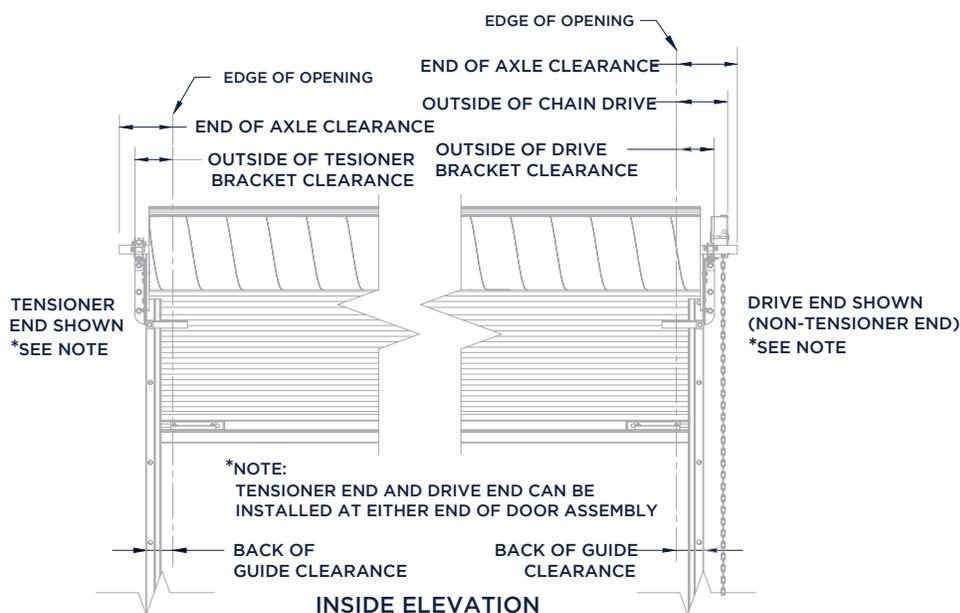
Universal mount 3" deep 12 gauge galvanized steel guides require no pre-installation modifications for wood, steel, concrete or filled masonry block applications.
