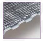
Insulation is made of a foil backed, dual layer of heavy-duty polyethylene air-bubble insulation secured in place with a strong adhesive and joined by mylar film to provide an R value of 4. (Top draft stop and side draft stopd are also included.)
