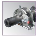
A cam-action spring tension holding device allows guick, easy and equal adjustment of the tension on all springs simultaneously from one end of the door. The cam tensioner bites into the axle helping to eliminate the unwanted spinning of the axle during the initial spring loading or adjustment process.
